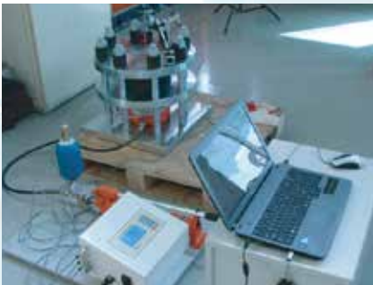
Creep Test Machine
