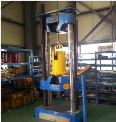
Variable Spring Hanger Performance Test
