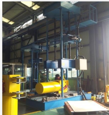
Constant Spring Hanger Performance Test
